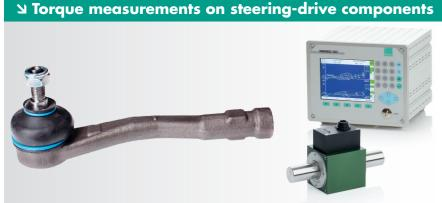
Steering rods, as a safety-related component, must undergo a defined test procedure both in pre-production testing and during the production process. After compression of the bearing, it is tested for low breakaway and friction torques. Torque sensor 8661 with 10 N\*m measuring range
