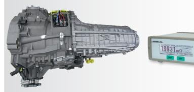
Very high accuracy is required for measuring the winding resistances of care must also be taken to make proper contact with the connecting electric motors. It is important that the three windings are symmetrical, studs to avoid contact resistances. and resistance values typically equal around 40 m $\Omega$ . In this situation,
