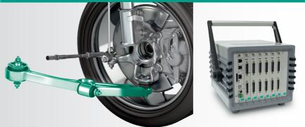
New developments in the motor industry involve comprehensive testing of safety-critical components such as control/suspension links. In these tests, strain gages are adhesively bonded to critical locations and readings taken by a high-speed measuring system. Versatile data recording
