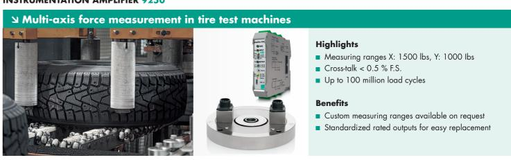
Vehicle tire testing places particular demands on our load cells. Measuother challenge is posed by the very large number of load cycles. In the rements must be acquired and analyzed simultaneously in two directions, event of a fault, maintenance staff must be able to replace the sensors X and Y, which demands low cross-talk between the two channels. The quickly and reliably to minimize down times.
