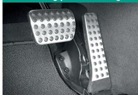
The actuating forces applied to pedals under different operating conditions are measured during test drives on the road and in the driving simulator to obtain a human/machine response profile and to determine the loads exerted on individual components. The sensor used in these ts has a low-profile design to minimize any impact on the feel
