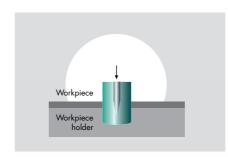
**RIGHT**: exact positioning of the part → avoids lateral forces and measurement
