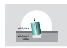
**WRONG:** Lateral forces → measurement errors can occur
