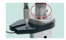
Ram with internal bore and grub screw
