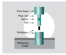
**RIGHT:** Press head, press ram, sensor, tool, workpiece and workpiece holder are precisely aligned with each other
