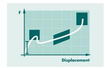
Force/displacement, e.g. when pressing a pin into a hole in the housing
