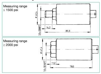
Tranducers with measuring ranges 10 psi and 15 psi have a diameter of 51 mm. Transducers with internal measurement amplifier are 26 mm longer and approx. 100 g heavier.
