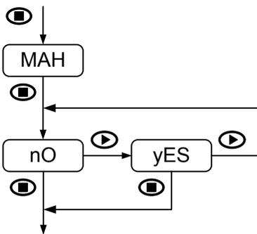
SHIFT key lock-out for MAX/MIN function is configurable in the same way as previous configurations.
