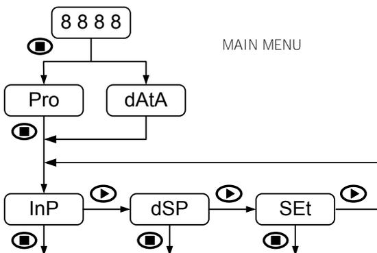
The instrument provides 3 keys for progressing through the menus and submenus and for data introducing/modifying:
