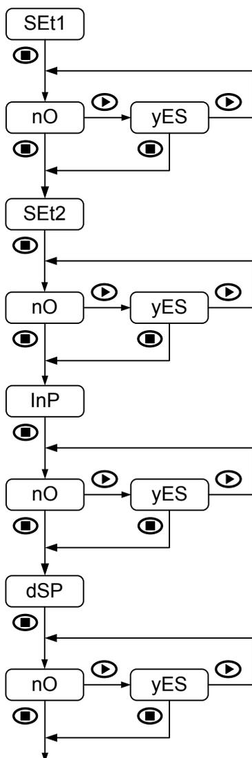
The following configuration access can be locked-out:
