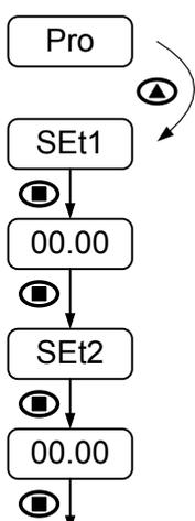
If 2RE output option is installed, it is possible to access to setpoints value configuration without having to enter main menu.
