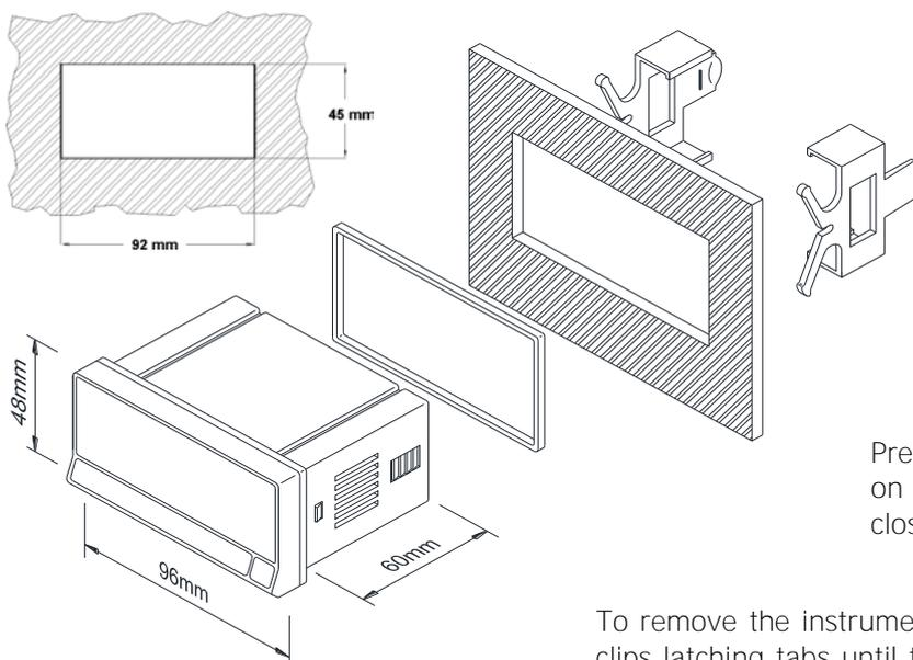
To install the instrument, prepare a 92x45mm panel cut-out and slide the unit inwards making sure of placing the sealing gasket between the front side panel and the frontal bezel.
