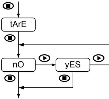
Access to TARE and TARE RESET functions activated through UP key can be blocked, as well.
