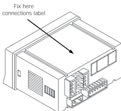
Once 2RE is installed and instrument is again inside the case, 2RE connectors should come out through the obtained orifice as this figure shows.
