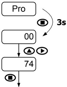
To access this menu from **RUN** mode, press **ENTER** key and while display shows "**Pro**" press again **ENTER** for at least 3 seconds.
