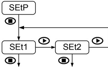
The third menu "SEtP" only appears when two relays output card is installed. For further details on function modes please refer to the corresponding **OUTPUT OPTION** part later on this manual.
