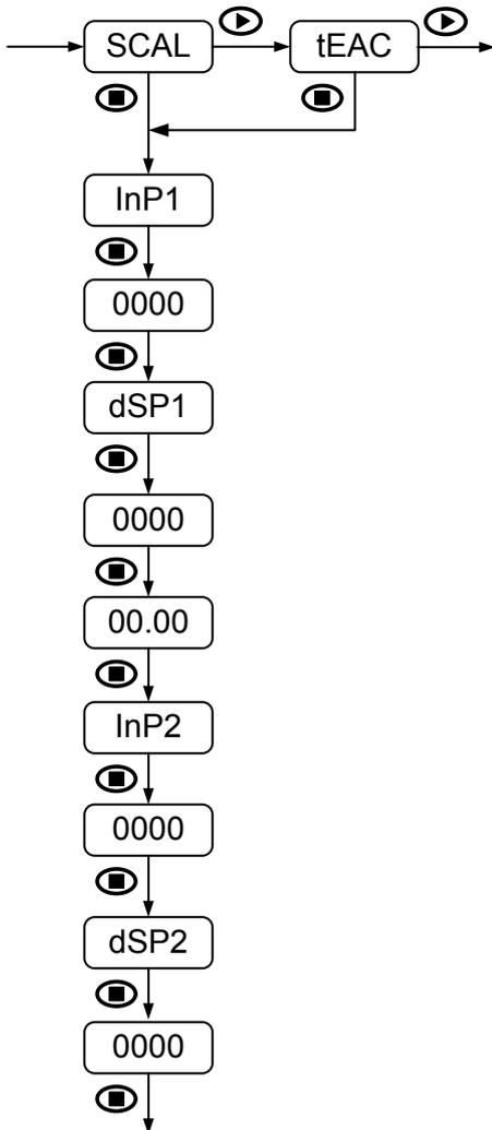
For both display scaling "SCAL" and "tEAC" methods, parameters to be sequentially introduced are identical.
